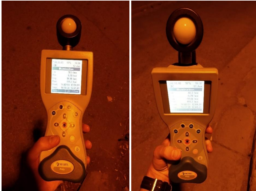
Image 42: Horizontal luminosity intensity measurement (left) and vertical luminosity intensity measurement (right)
