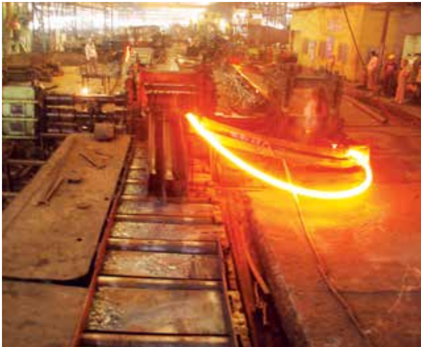
Figure 1 Steel being rolled into a TMT bar in a re-rolling mill
