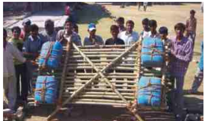
Use of Locally Available Materials for Making Tarapa
